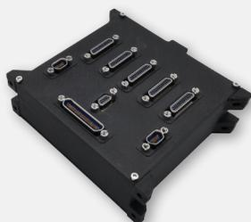
The RPCU/RPDU is provided with two independent circuits (primary and secondary), based on two different (in density and reliability) FPGAs. In nominal conditions the primary circuit implements the data routing among the cameras and between the cameras and the spacecraft. The secondary
